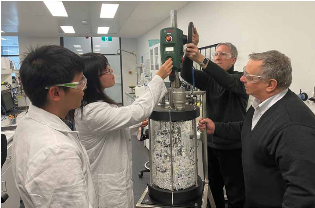
Recycling 'wash reactor' mini-rig, tests label and glue variations to improve recyclability (UNSW).
